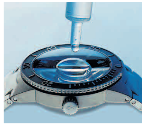
After the pressure test, the candidates are heated. If the watch isn’t hermetically sealed, then a drop of cold water placed atop the crystal will cause a droplet of water to condense on the underside of the sapphire pane.
