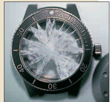
This Aquatimer failed its 200-bar pressure test. The watch’s 3.7-mm-thick crystal shattered. Sometimes the tiniest hairline faults, invisible to the naked eye, are enough to doom a crystal.
